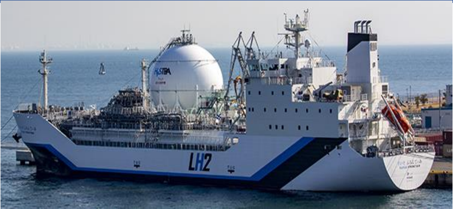
KHI, Suiso Frontier (2021) Spherical tank, 1250m 3
